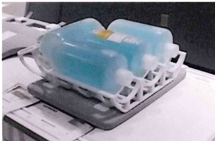
Figure 15: Phantom position in coil. Coil flat on table.
