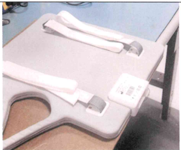
Figure 3: Location of coil label on the PROCURE coil.
